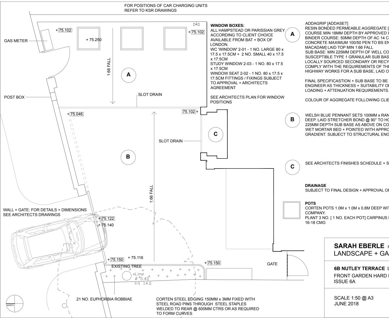
RESIN BONDED PERMEABLE AGGREGATE [ 6 OR 10MM ] SURFACE COURSE MIN 18MM DEPTH BY APPROVED INSTALLER. BINDER COURSE: 50MM DEPTH OF AC 14 CLOSE SURF ASPHALT
