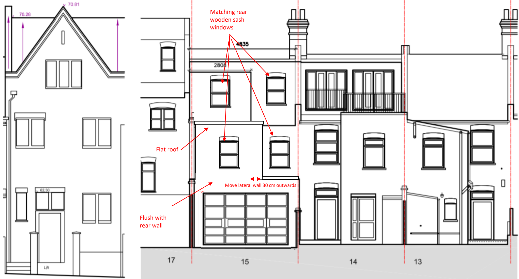
02. Back Garden Elevation (North Elevation)
