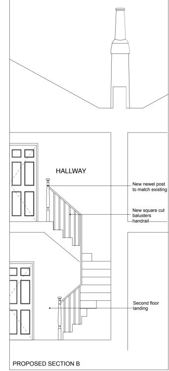
Balusters, handrail and nosing details all to match existing staircase
