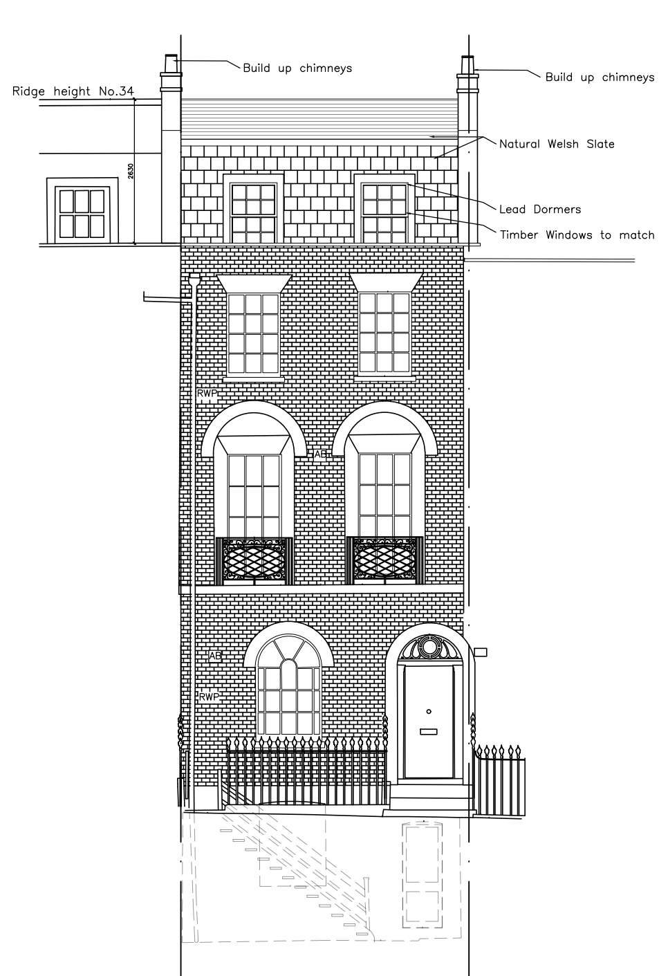
Proposed Front Elevation SCALE 1:100
