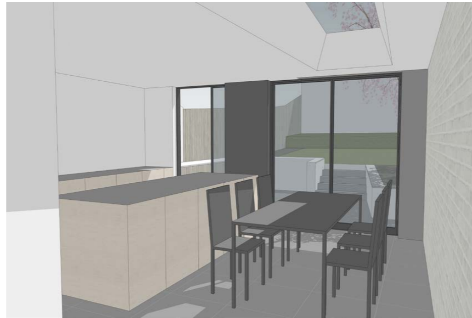
Flat ceiling with rooflight
