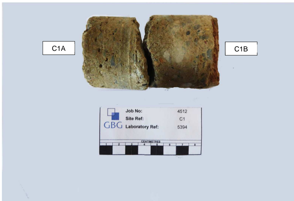
Concrete Core Sample (C1) extracted from 1 st Floor Deck.
