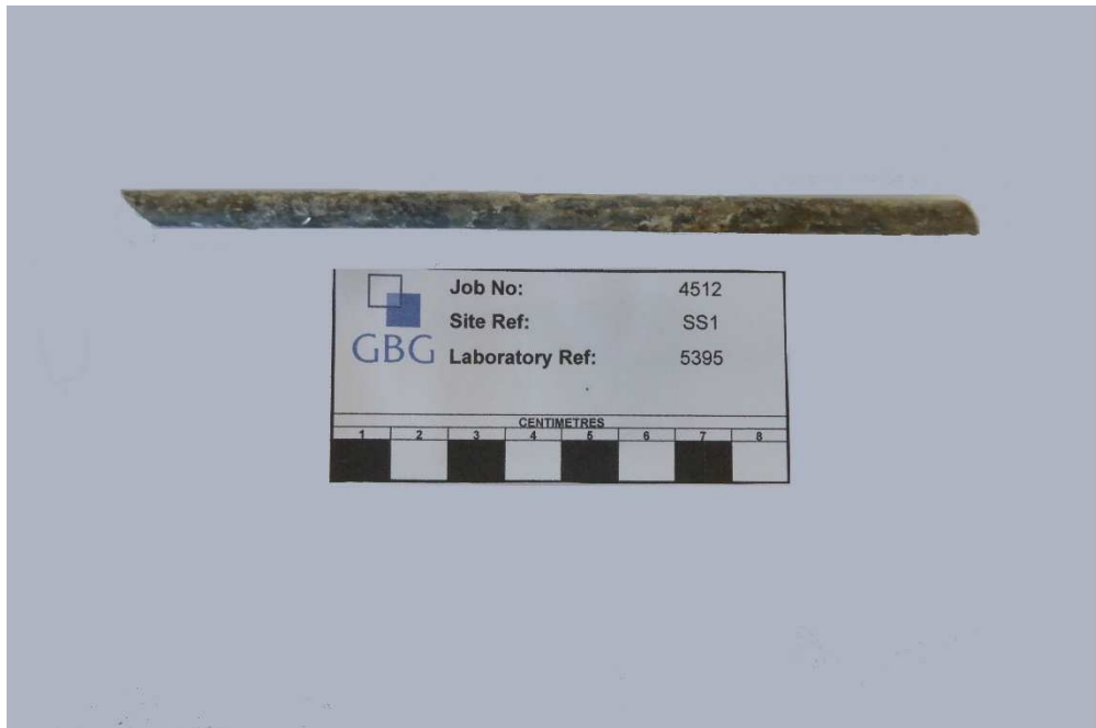
Steel Reinforcement Sample (SS1) after extraction
