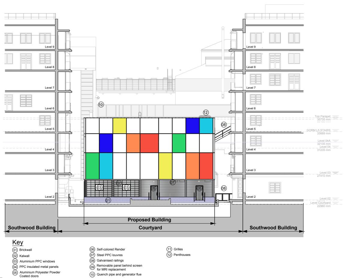
(10) Quench pipe and generator flue
