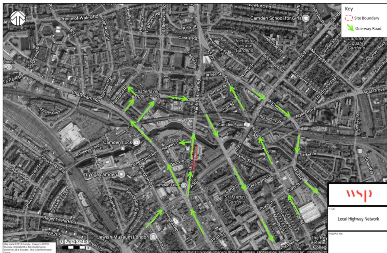
Figure 4-2: Local Highway Network One-way System
