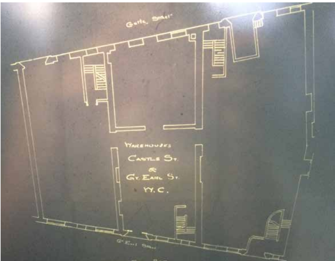
10b. First floor plan showing the 1907 conversion of the Seven Dials Warehouse (CLA)
