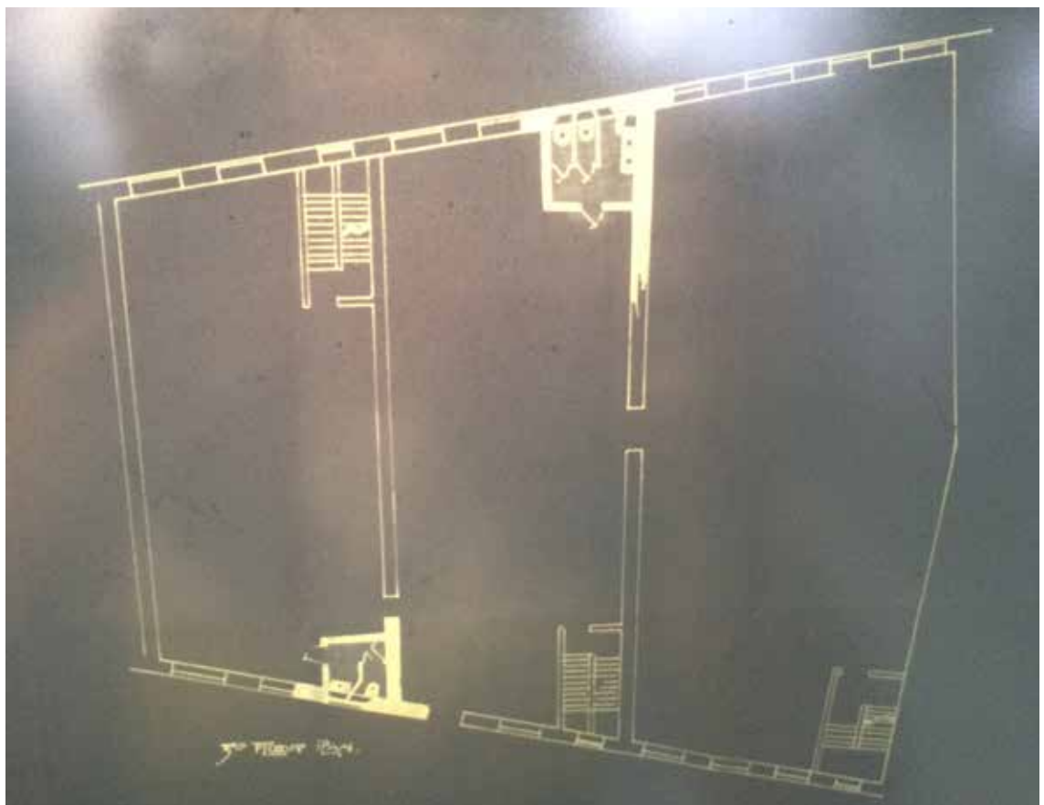
10d. Fourth floor plan showing the 1907 conversion of the Seven Dials Warehouse (CLA)
