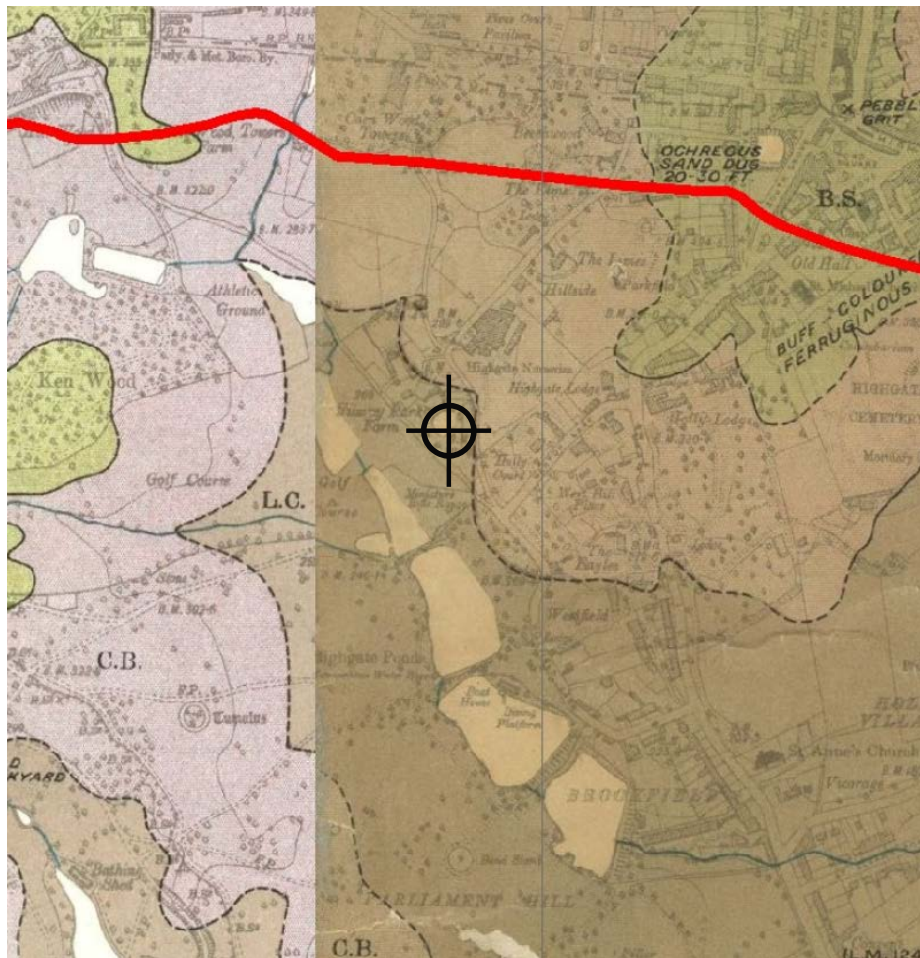
Camden 1920 Geological Map (Figure 2, CGHHS, 2010) (London Clay is shown to underlie the site)
