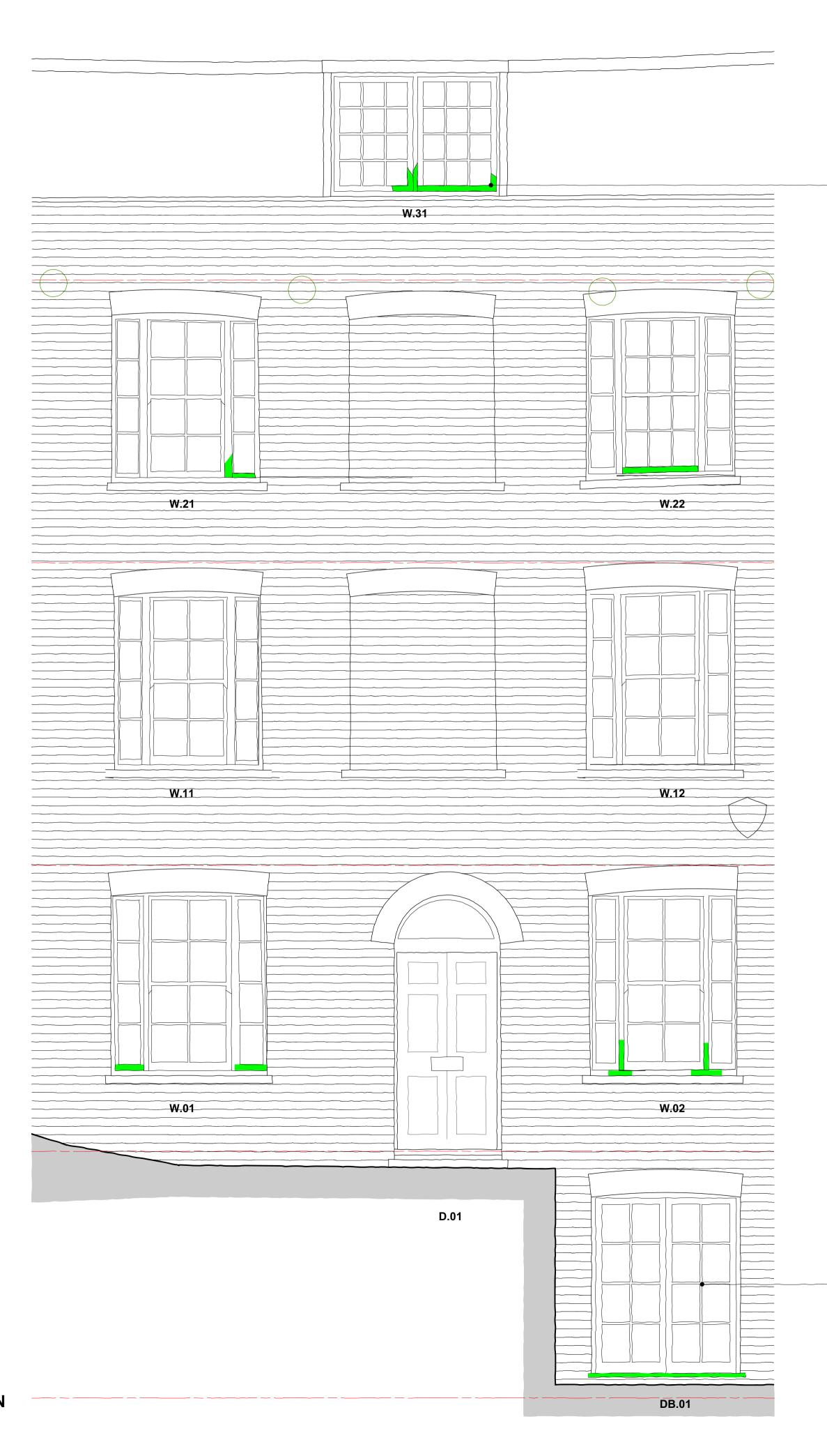
Replace bottom rail where indicated. Cut back existing damaged timber to ensure new timber sections are spliced into sound timber (mullions and
