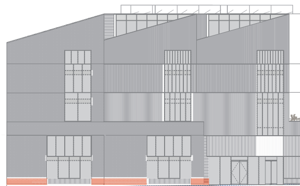
3 - Lower level concrete upstand
