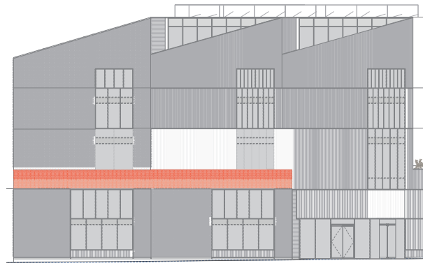
2 - Horizontal brickwork band
