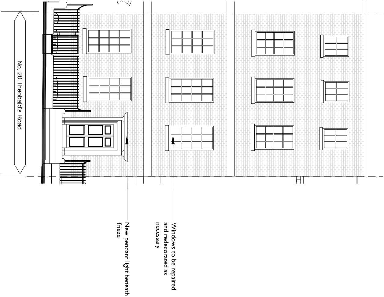
02 FRONT ELEVATION AS PROPOSED 409 1:100 @ A3
