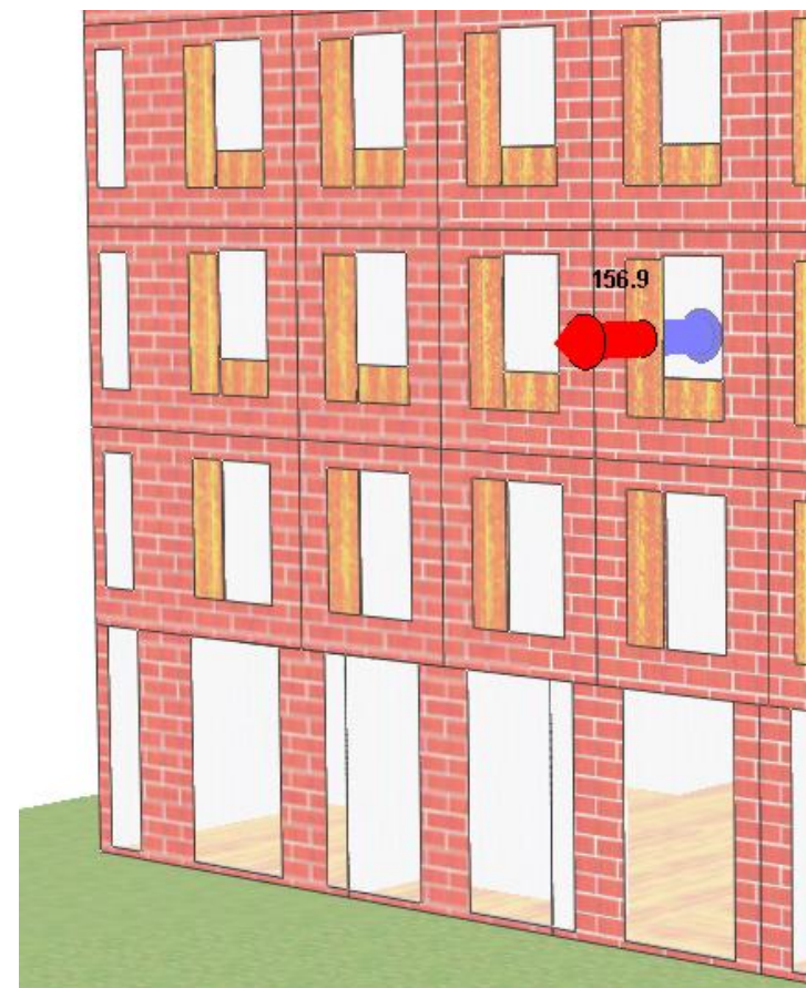
Figure 3.1.3 Figure to show the inlet and outlet flow of natural ventilation for a bedroom
