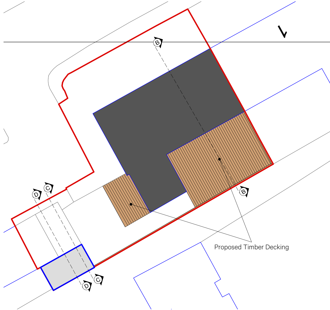
Location of Proposed Garden Timber Decking - 1 : 200
