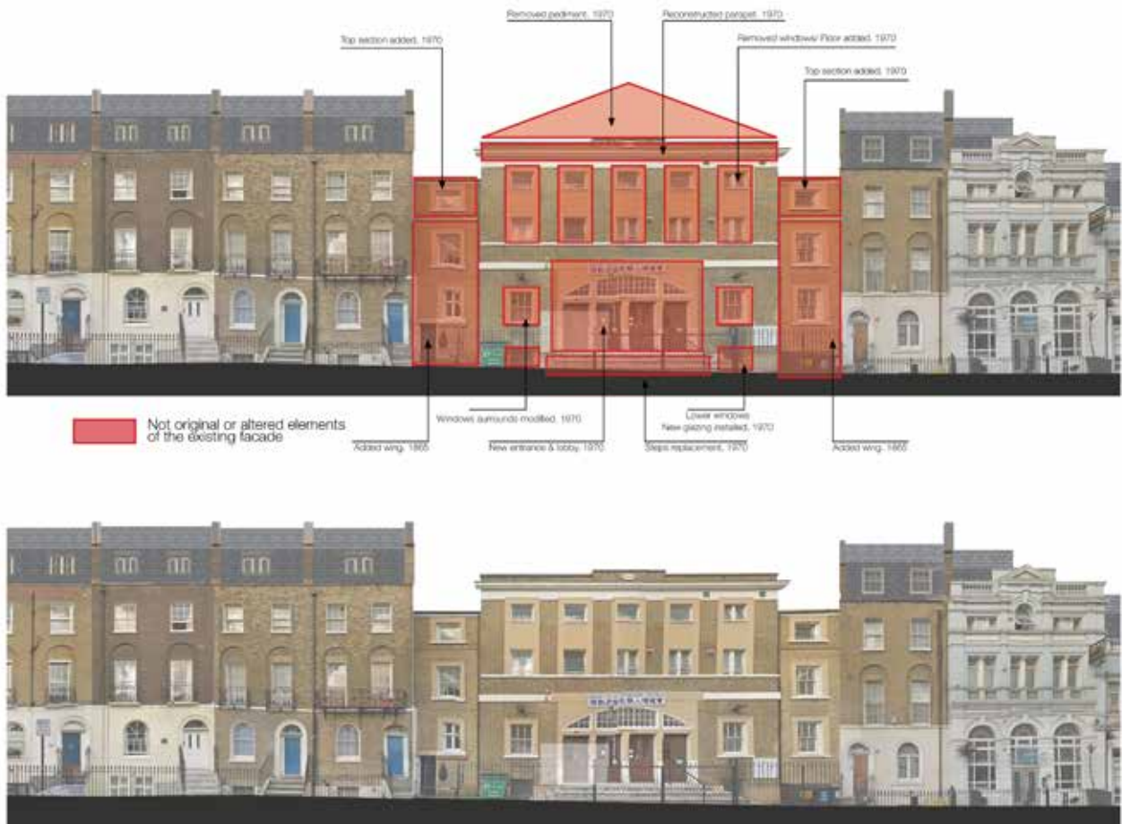
Birkenhead Street existing elevation. Altered, lost or additional areas to original shown in red (Dexter Moren Associates)
