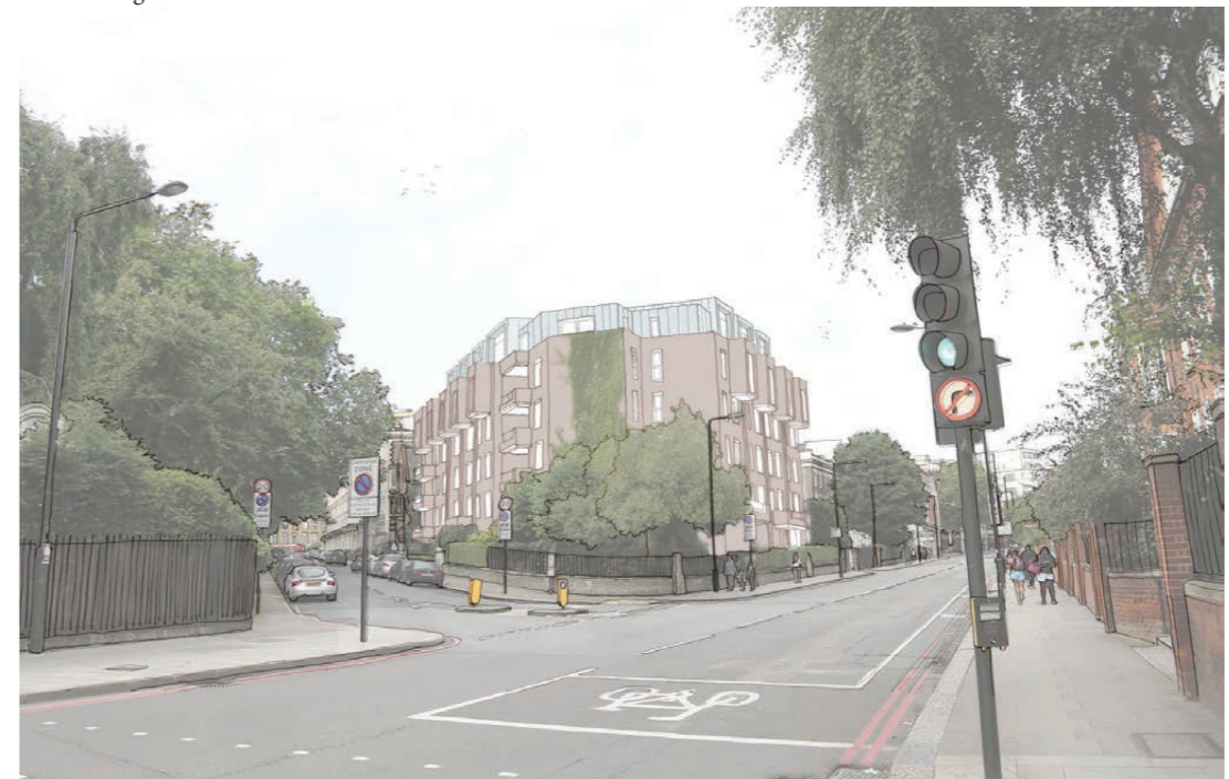
Stage 4: Developed black and white image scanned and imported into photoshop allowing the sketch to be correctly positioned back over the photo in stage 1. The process creates an artistic view which is accurate in terms of context, perspective and scale with a colour wash applied to indicate proposed materials.
