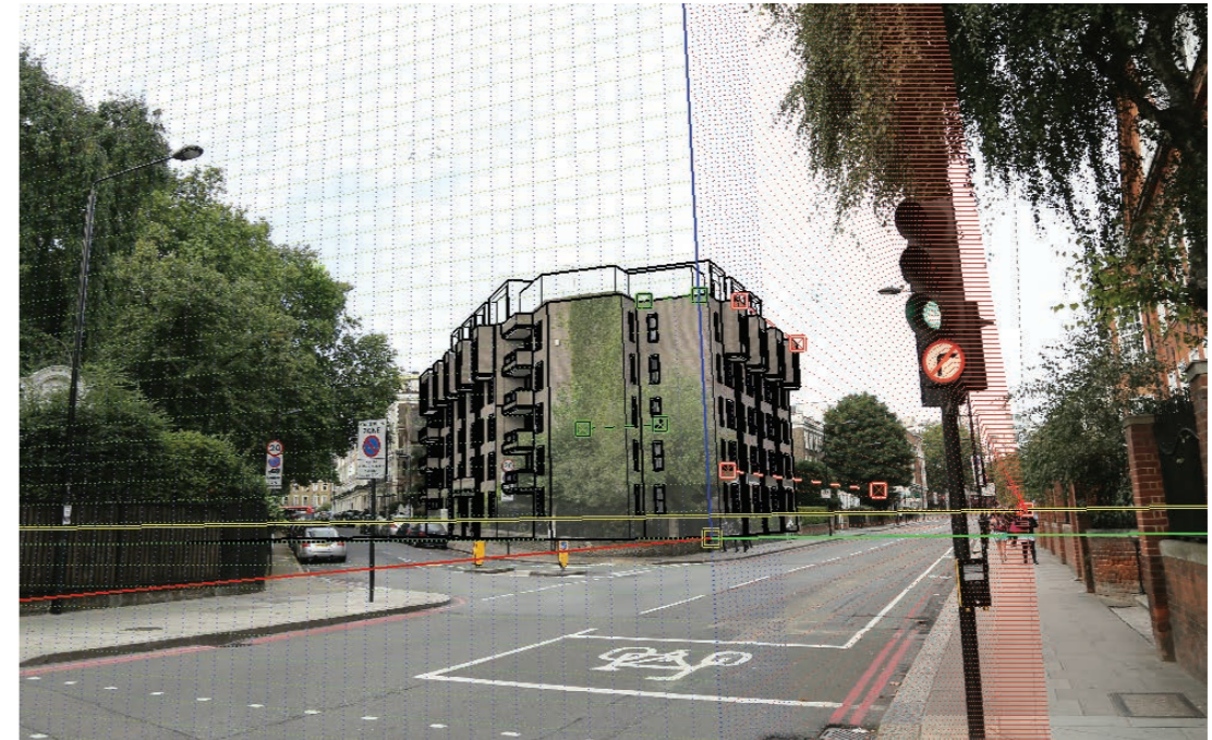
Stage 2: 3D Sketch up model constructed to scale including the surrounding context, existing building and proposed roof extension. The model has been adjusted using the photo match tool to position the model in the correct perspective to the photograph taken in stage 1.
