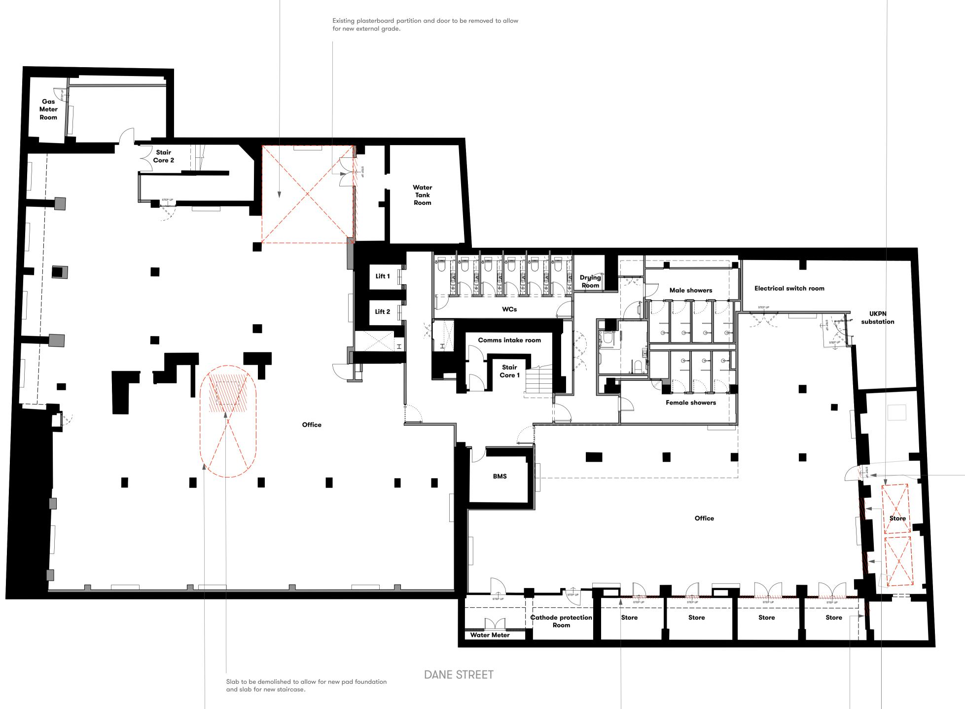
Slab to be demolished above to create new internal opening with new downstand supporting structure to opening perimeter, to Structural Engineer's details.
