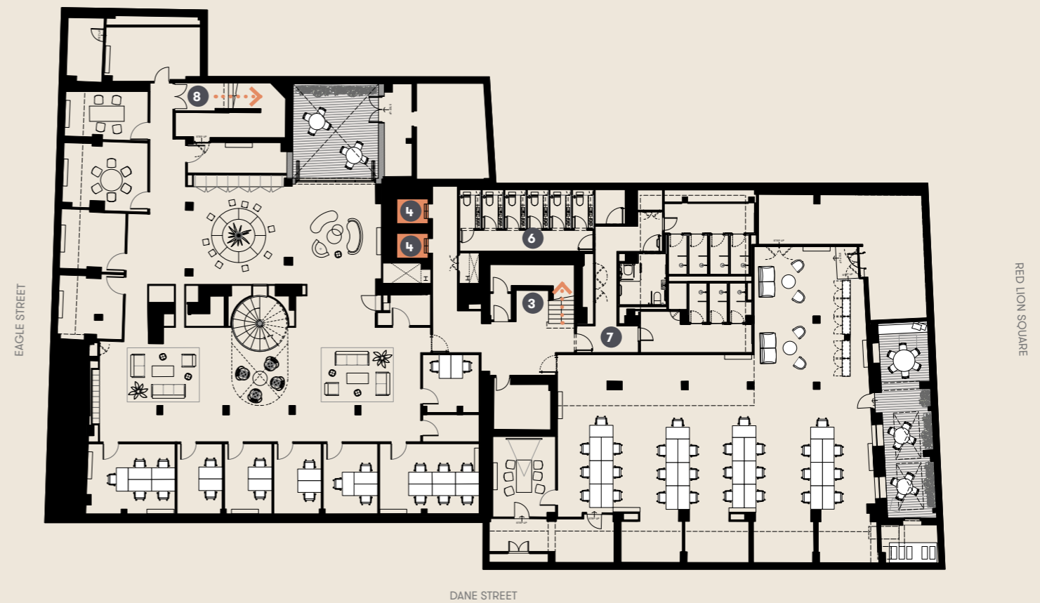
7.1B Lower Ground Floor Access Arrangement
