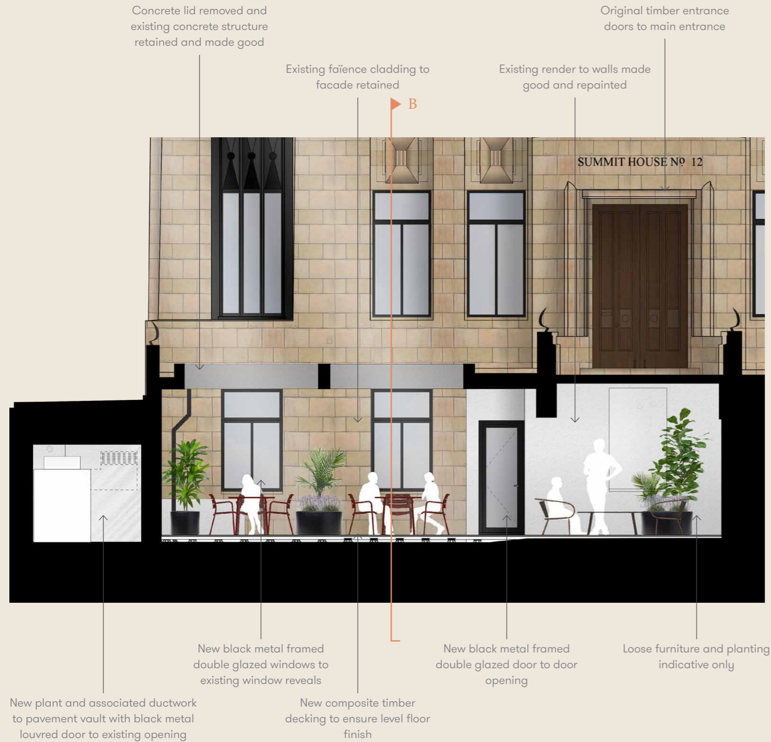
6.4.C Proposed Sectional Elevation A through light well
