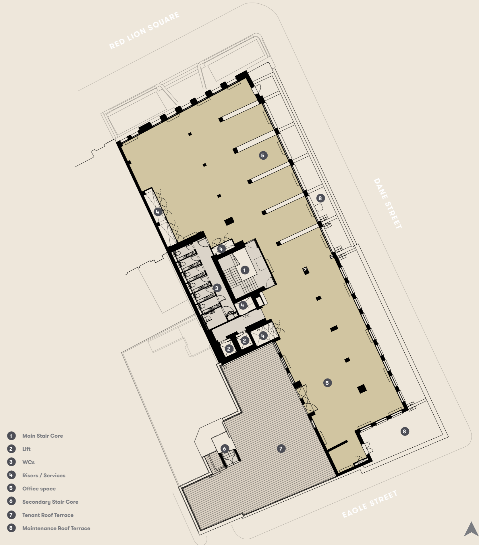
5.4.D Existing Fourth Floor Arrangement
