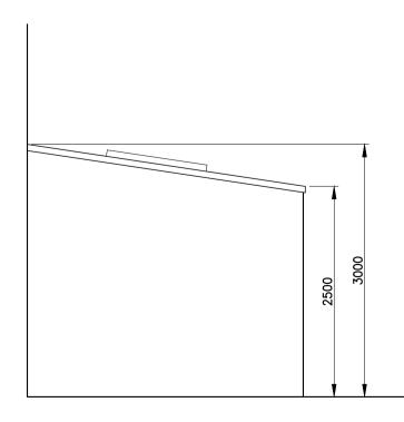
Proposed Rear Extension Flank Elevation
