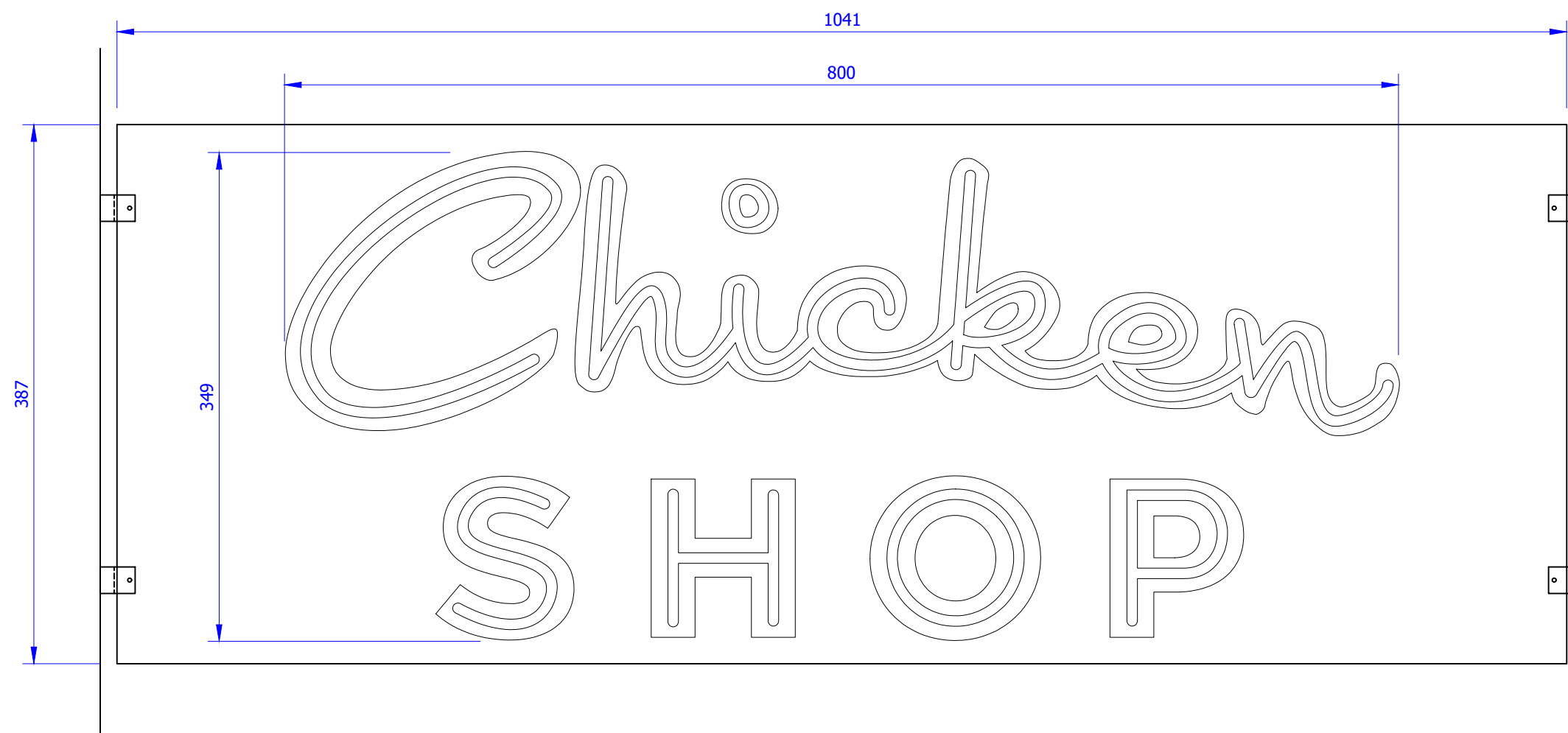
Elevation View Faux neon letters 1no Faux neon White mounted to 3mm flat aluminum letter shapes finished Blue PMS 646, all mounted to suspended clear 5mm acrylic panel. To be mounted behind glass with Shopkit fixtures side mounted to brick wall. scale: 1:4
