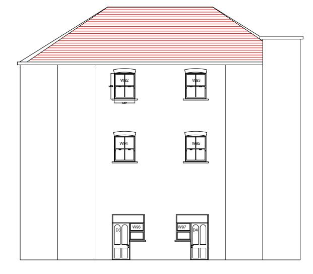
Proposed are replacement for single glazed sash window to like for like timber slim-lite Double glazed sash window.
