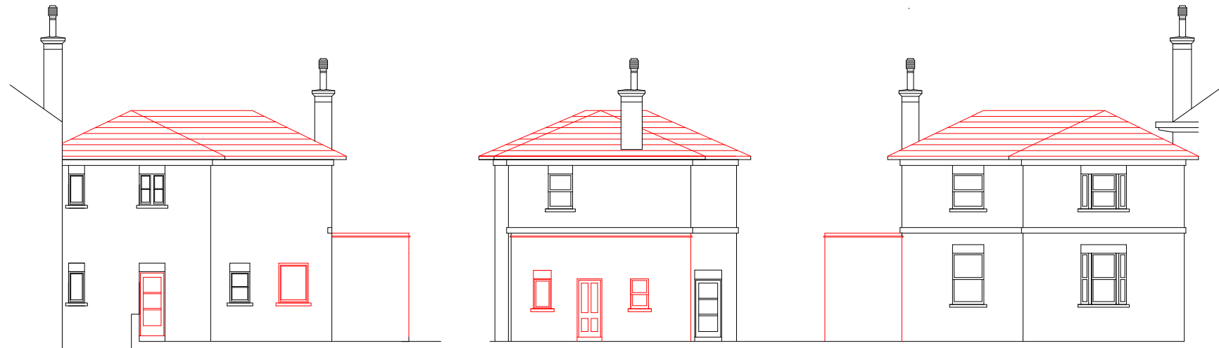
EXISTING ELEVATIONS - RED SHOWS DEMOLITIONS
