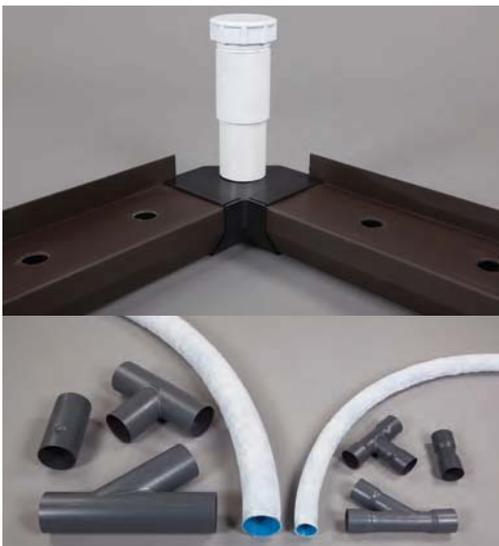
**Delta Channel** is a water collection conduit which is bedded into a preformed channel at the floor/wall angle. Holes in the channel wall allows water to ingress at this point to drain away to a sump or soak away. Access ports are available to allow maintenance and inspection. The system is joined with a range of connectors.
