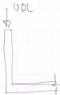
$$@ U = \left( 1.5 \times \frac{6}{2} + 1.5 \times \frac{3.7}{2} + 0.6 \times \frac{3.7}{2} \right) \times \frac{4.7}{2} = 19.7 \text{ kN.}$$
