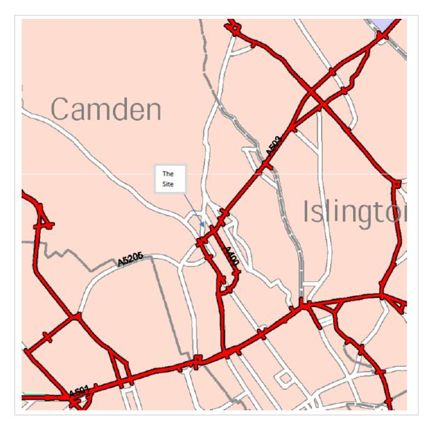
The site is located immediately to the north of the TLRN as shown in the figure above. The routes used to travel to and from the site are one-way roads. Vehicles will approach the site from the south via Camden High Street (A400), part of the TLRN, or from the south west via Parkway (A4201). Vehicles will leave the site via Kentish Town Road (A400). These routes are shown in the figure below together with the routes from/to the TLRN.
