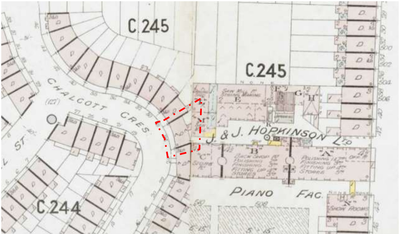
Figure 11: 1900 Insurance Plan of London North West District Vol. C: amalgamation of sheets 28 and 29. No. 26 Chalcot Crescent (red dash) can be seen directly abutting the Hopkins Piano Factory buildings. Note the maps provide scale and material annotations for all masses. Source: British Library Online Gallery (accessed 20 th September 2018). Adapted from: http://www.bl.uk/onlinegallery/onlineex/firemaps/england/london/atoc/zoomify151903.html http://www.bl.uk/onlinegallery/onlineex/firemaps/england/london/atoc/zoomify151904.html
