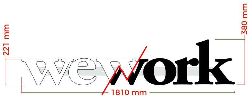
Sign 3 - 1 Set of Built up internally illuminated logo letters (Day/Night acrylic) fitted above window (Lux level 300 cd/m)
