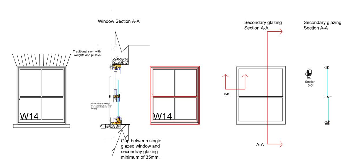
Existing single glazed timber window to be exactly same to keep the heritage look of the building and new secondary glazing to be fitted for thermal proposes to stop condensation and noises Notes:
