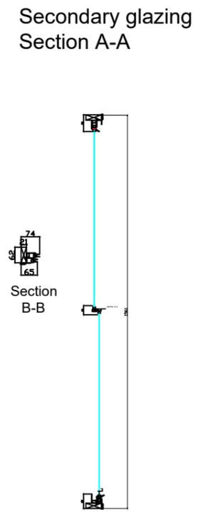
Gap between single glazed window and secondary glazing minimum of 35mm.
