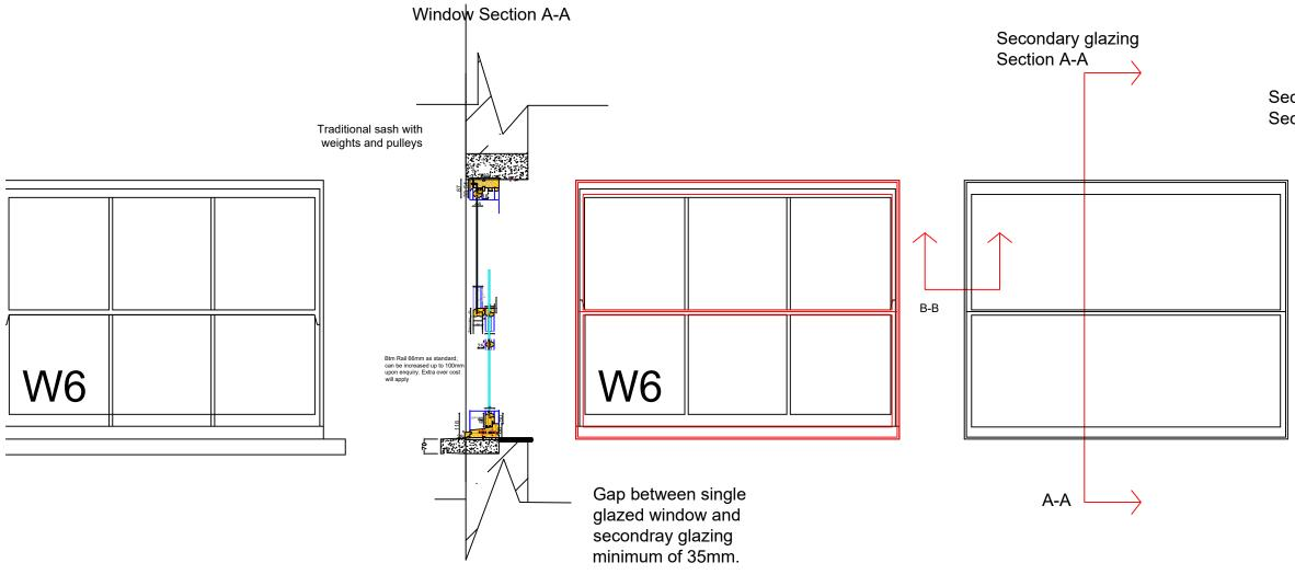
Existing single glazed timber window to be exactly same to keep the heritage look of the building and new secondary glazing to be fitted for thermal proposes to stop condensation and noises
