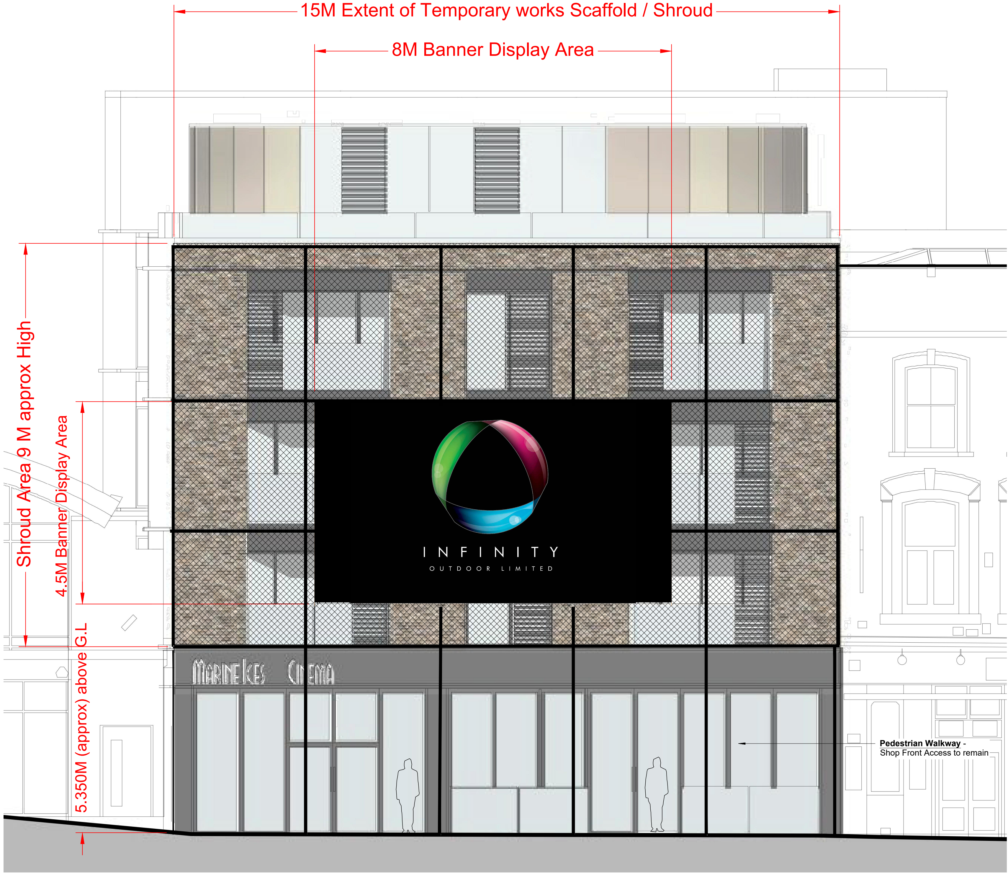
Proposed Front /South West Elevation / Haverstock Scale 1:50
