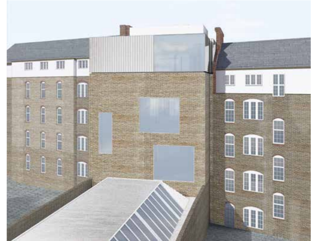
03 Single stair landing window, with larger misaligned openings to the office floor.
