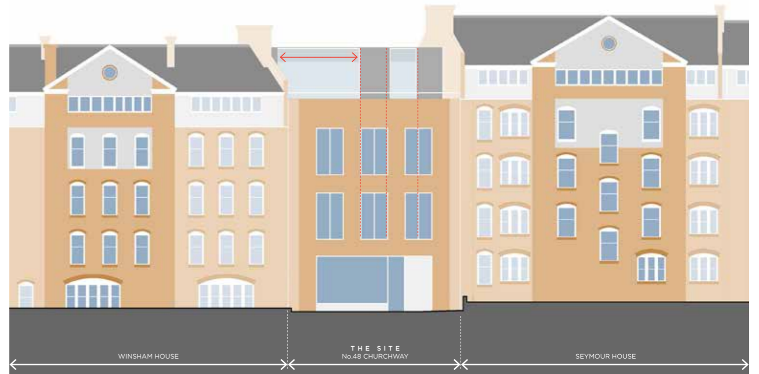
06 Asymmetrical alignment to the upper set back apertures and increased generosity to size of openings.
