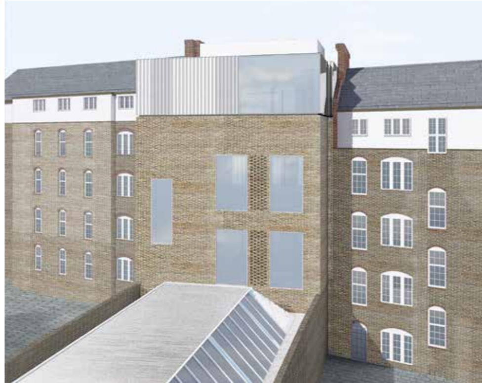
02 Single stair landing window and aligned upper stair window, with vertically aligned window openings to office floors. 'Hit and miss' brickwork to first and second floor, and perforated metal cladding to third provide natural venting to the offices.
