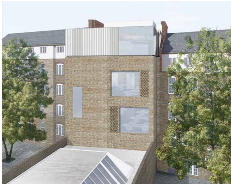
05 Single stair landing window and aligned upper stair window, with larger, misaligned recessed openings to the office floors. 'Hit and miss' brickwork to first and second floor, and perforated metal cladding to third provide natural venting to the offices.
