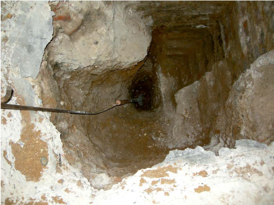
Fig 15 A photograph of a geotechnical test pit observed in the basement level of 18–21 Hand Court, showing foundations and natural gravel deposits. MOLA photo 2017
