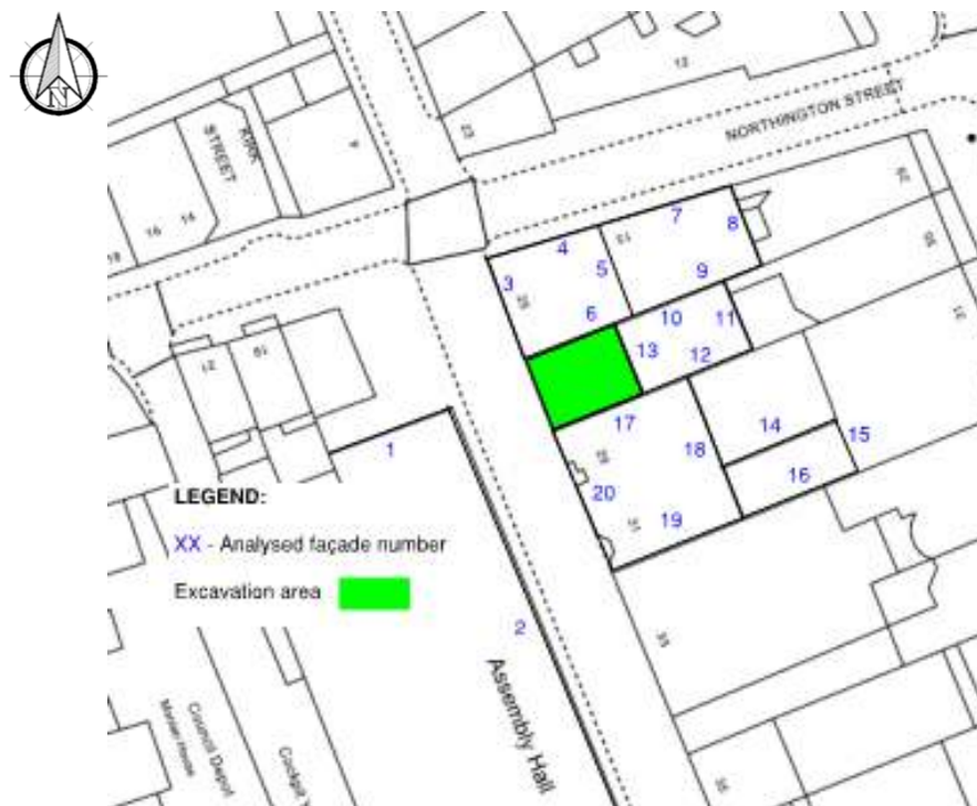
Figure 4.3 Simplified scheme and nomenclature for each building façade/masonry wall element. Green area depicts approximate location of the excavation.
