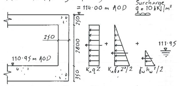
Assume: - 250 mm thick propped retaining wall
