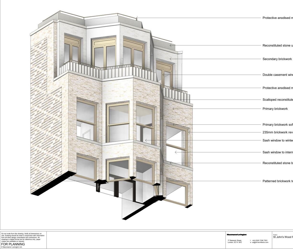
Protective anodised metalwork railing
