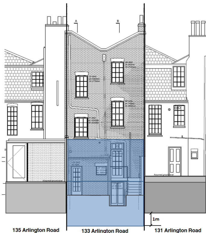
Section (A-A) drawing showing proposed rear extension (blue) against the assumed extent of the existing adjacent extensions
