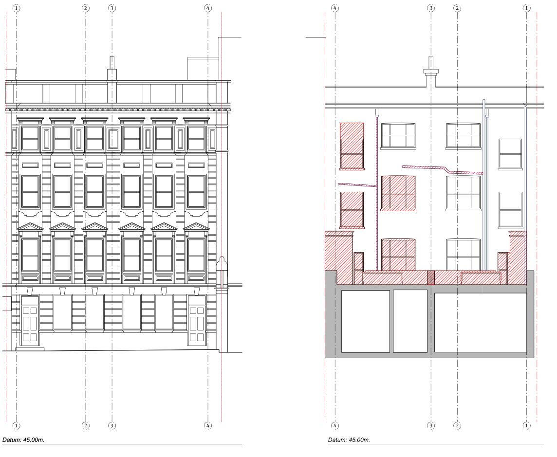
Existing Front & Rear Elevation / Section AA Demolitions Project No. Date Scale SK1302 01/03/13 1:100 @ A3
