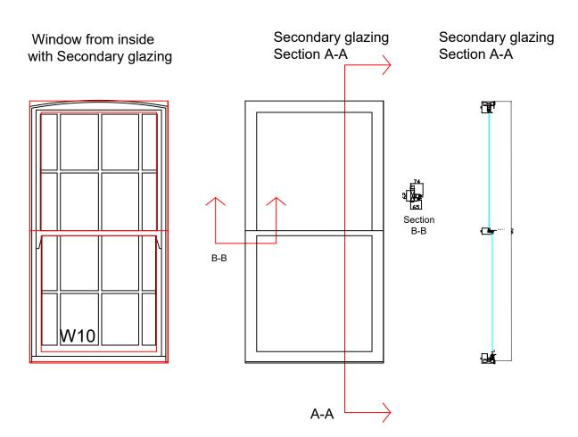
Existing single glazed timber window to be exactly same to keep the heritage look of the building and new secondary glazing to be fitted for thermal proposes to stop condensation and noises
