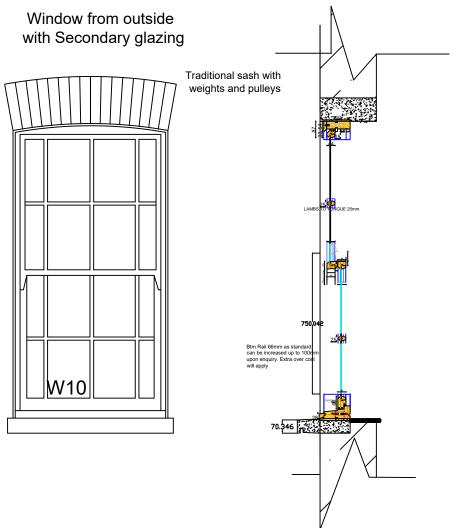
Gap between single glazed window and secondray glazing minimum of 35mm.
