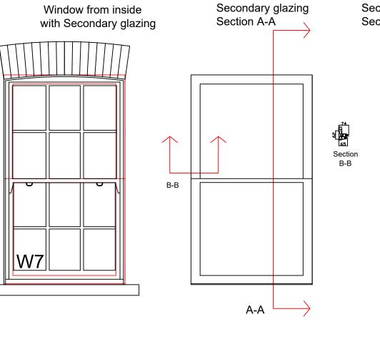
Existing single glazed timber window to be exactly same to keep the heritage look of the building and new secondary glazing to be fitted for thermal proposes to stop condensation and noises
