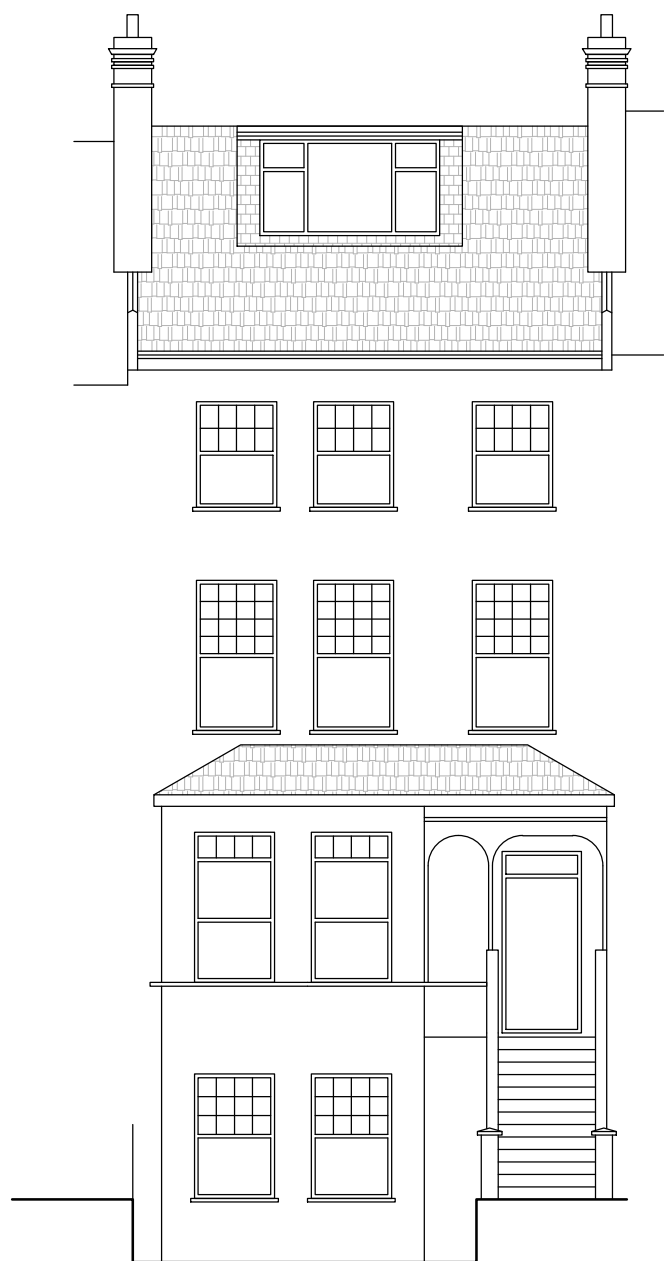
FRONT ELEVATION (ALL WINDOWS TO MATCH EXISTING)
