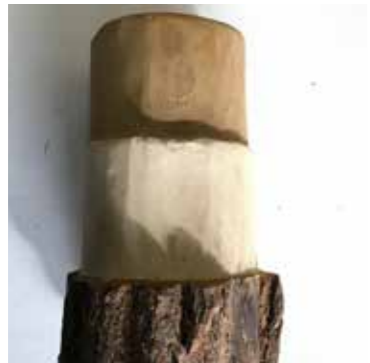
Robinia posts (bark and sap wood removed)
