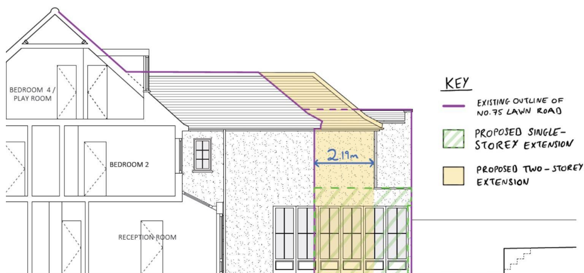
Extract from section B-B showing extent of 2-storey pitched rear extension in relation to existing property outlines in purple.
