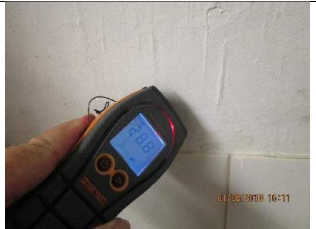
High levels of up to 46.3% moisture were recorded to the walls surfaces, as indicated
