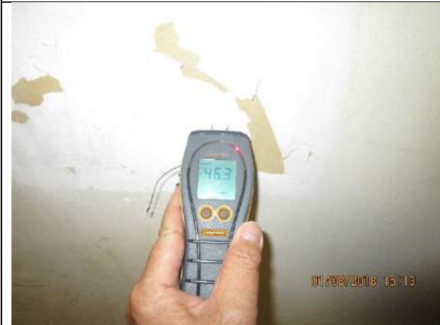
High levels of up to 46.3% moisture were recorded to the walls surfaces, as indicated
