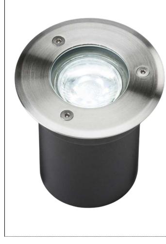
Material: Stainless Steel Voltage: 230V IP Rating: IP65 Lamp Wattage: 3Watt No. LEDS: 9 Lumen Output: 290Lm Lm/W (Efficiacy): 82Lm/W Lamp Colour: 6000K Beam Angle: 35degrees Dimensions: Diameter 92mm Cutout 61mm Height 97mm
