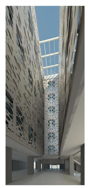
Use of colour mood lighting, behind the perforated screen as part of the wall, will enhance the space giving the option of subtly reducing the light in the atria during the night and increasing light into this central area on dark overcast days.
