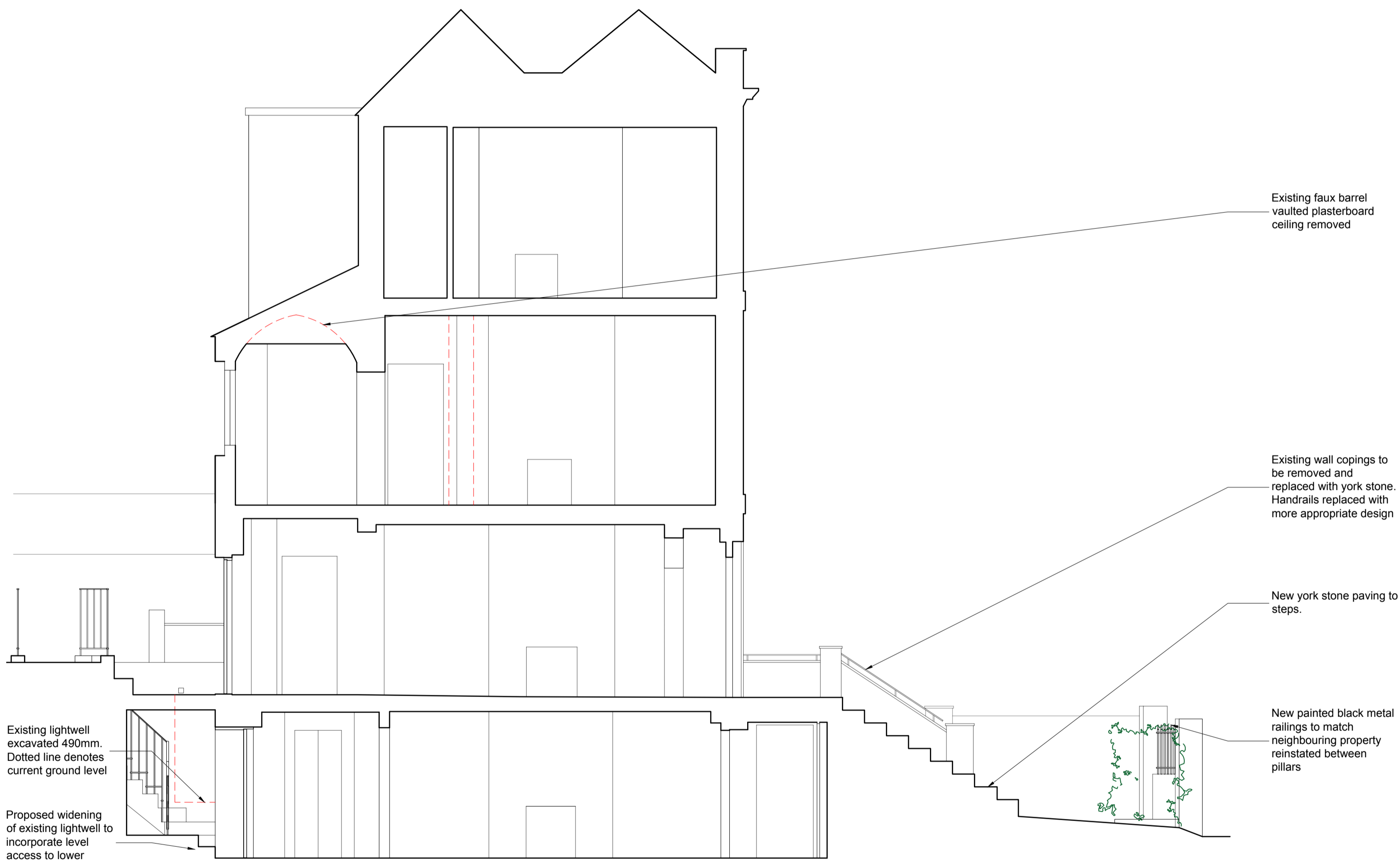
Existing Section A-A
